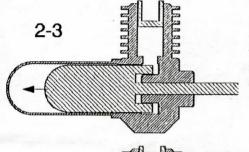
In the second phase the working piston has been pushed outwards thus giving the air a bigger volume and reducing the pressure in comparison to the first phase.
