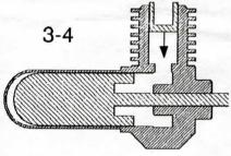
In the third phase the displacer is moved to the front end position causing the hot air to be displaced from the hot area of the motor towards the cold end of the motor. In the cold area and at the walls of the displacer heat is transferred from the air which causes the air to be cooled down and reducing the pressure inside the engine.
