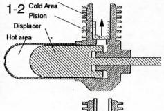
piston in the inner end position. The air in the hot area of the engine is heated up, which causes the internal pressure in the engine to rise. The resulting pressure is transmitted to the area of the working piston and causes it to be pressed outward. Thus work is extracted.
