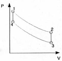
A graph of the pressure and volume of the ideal Stirling cycle is shown to the left. Process 1-2 is the isothermal expansion, where mechanical work is extracted. Process 2-3 represents the constant volume cooling. Process 3-4 is the isothermal compression of the working medium, process 4-1 is the constant volume heating, which completes the cycle.
