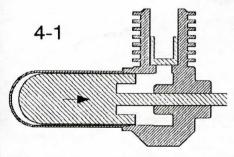
In the fourth phase the piston is moved into the inner end position, which has been made possible by the reduced internal pressure. Simultaneously the air is compressed, the required energy is supplied by the flywheel. Then the diplacer is moved again into the inner end position causing the air to be transferred from the cold area to the hot area,
